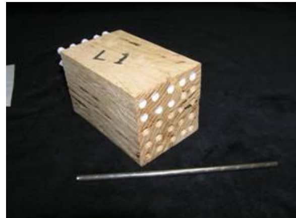
Release paper, it unrolls to fill hole
